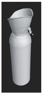
Figure 4: CT projection of oxygen boost can
