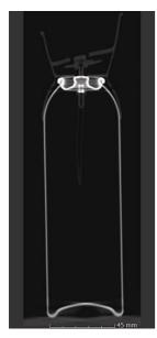
Figure 5: Right slice of oxygen boost can
